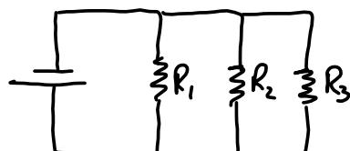
In a parallel circuit, the current is divided (split) between the resistors. The potential difference across each resistor is the same.
