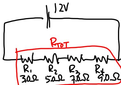
a) Series:  $R_{TOT} = 3.0\Omega + 5.0\Omega + 7.0\Omega + 9.0\Omega$
