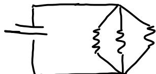
$$\frac{1}{R_{TOT}} = \frac{1}{R_1} + \frac{1}{R_2} + \frac{1}{R_3} + \dots + \frac{1}{R_N}$$
